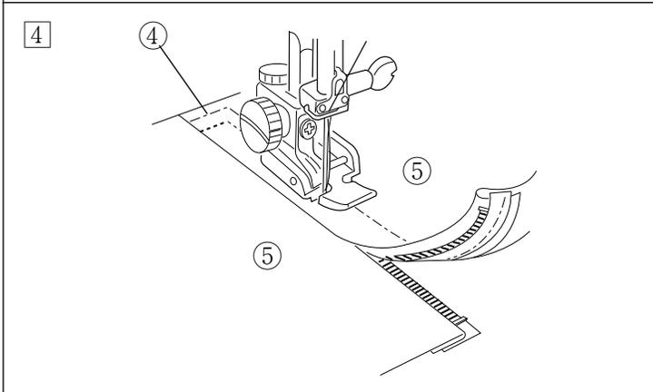
4 Move the zipper foot to the left pin. Guide the edge of foot along the zipper teeth and stitch through the garment and zipper tape. Stop about 5 cm (2") from the top of the zipper.
