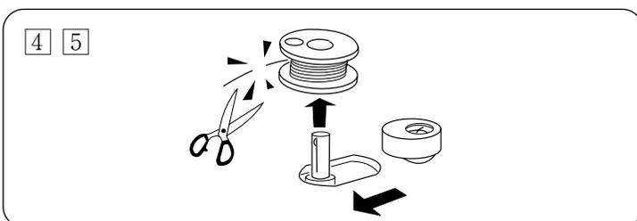
④ Depress the foot control again. When the bobbin is fully wound, it will stop automatically.
