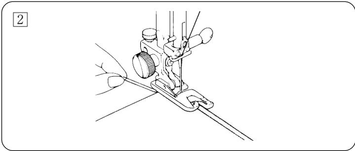
2 Lower the needle into the fabric at the point where sewing is to begin and lower the hemmer foot. Sew 3 or 4 stitches while holding the needle and bobbin threads.
