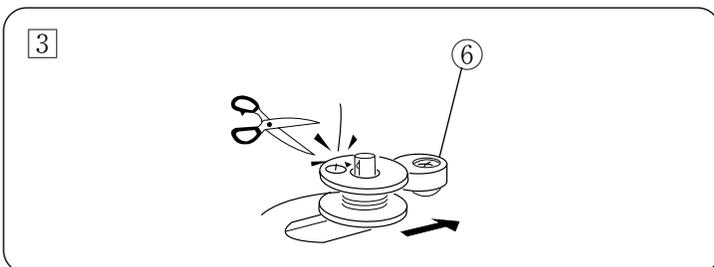
③ Put the bobbin on the bobbin winder spindle and push it to the right. With the free end of the thread held in your hand, depress the foot control. Stop the machine when it has made a few turns, and cut the thread close to the hole in the bobbin.
