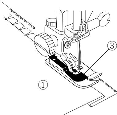
Position the fabric so that the folded edge comes to the left side of guide. Lower the presser foot. Adjust the position of needle swing with the stitch width key so that the needle just pierces the folded edge of the fabric when the needle comes over to the left side. Sew guiding the folded edge along the guide. For a professional looking hem, fold the fabric reducing the width to about 0.2 cm (1/8"). As you sew, the right hand stitch will fall off the fabric edge forming a chain stitch.
