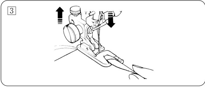
3 Lower the needle into the fabric and lift the hemmer foot. Insert the folded portion of the fabric into the curl of the hemmer foot.
