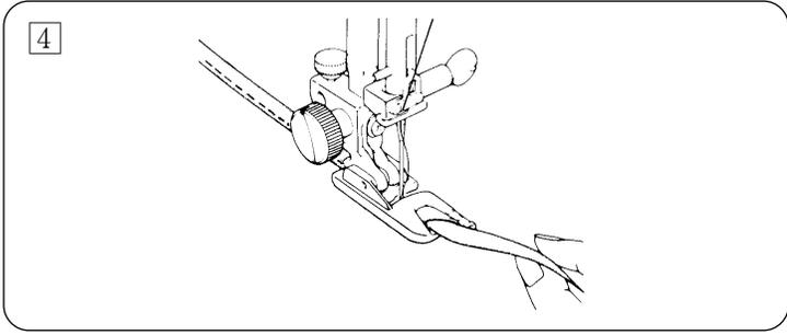
4 Lower the hemmer foot, then sew by lifting up the edge of the fabric to keep it feeding smoothly.
