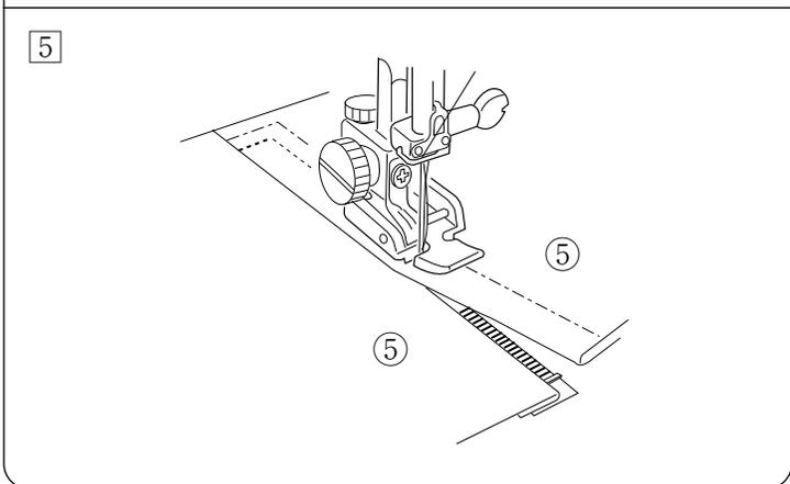
5 Lower the needle slightly into the fabric, raise the foot, remove the basting stitches and open the zipper. Lower the foot and stitch the remainder of the seam, making sure the fold is even.
