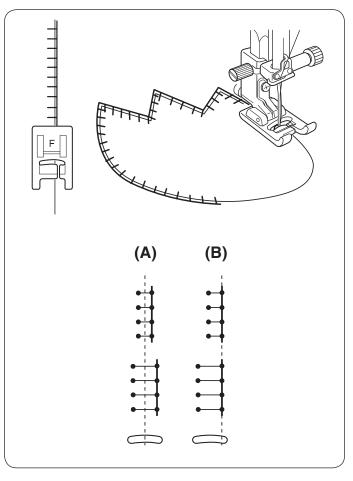
Place an applique on the fabric and baste it in place or use a fusible web to secure the applique in place. Guide the applique fabric, so that the needle falls off the edge of the applique when the needle swings to the right.
