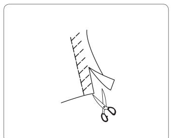
Place your fabric to allow a  $5/8^{\circ}$  (1.5 cm) seam. Trim excess close to the stitching. Be careful not to cut the stitches.
