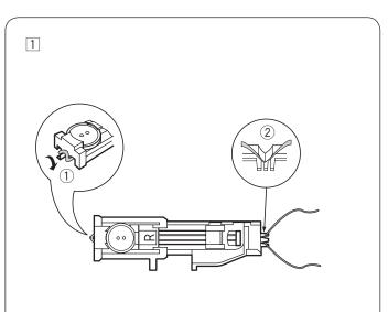
Use the same procedure as the square buttonhole procedure. Set the stitch width to match the thickness of the cord used. With the buttonhole foot raised, hook the filler cord on the spur ① at the back of the buttonhole foot.
