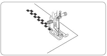
For a delicate appearance on fabric such as chiffon, use a single layer with a tear-away backing, if necessary.
