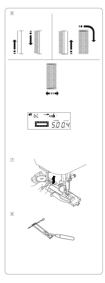
6 The buttonhole is sewn automatically in the sequence shown. When the buttonhole is finished, the machine will stop automatically with the needle in the up position.
