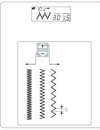
Zigzag stitch is used for various sewing needs including overcasting. It can be used on most woven fabrics. A dense zigzag stitch can also be used for applique.
