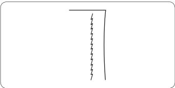
This is a narrow stretch stitch in the left needle position designed to eliminate puckering on knit fabrics and bias seams, while permitting the seam to be pressed completely open flat.
