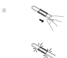
3 Pull the loose ends of the filler cord to tighten it.
