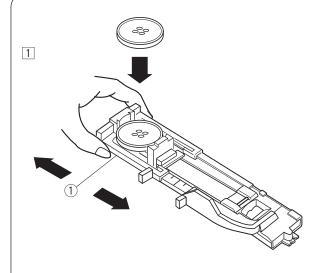
The size of a buttonhole is automatically set by placing a button in the rear of automatic buttonhole foot R.
