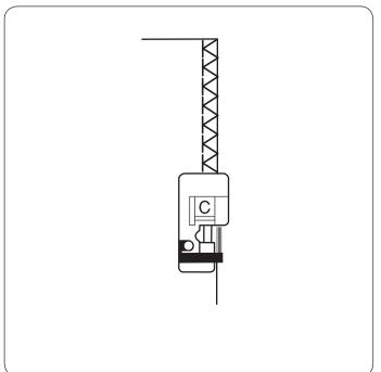
This stitch can be used to simultaneously seam and overcast edges of fabrics.
