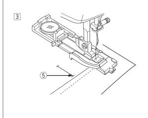
The size of a buttonhole is automatically set by placing a button in the rear of automatic buttonhole foot R.
