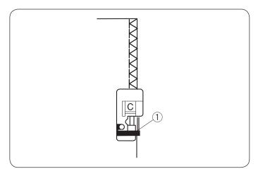
This stitch is used to seam and overcast fabric edges at one time.
