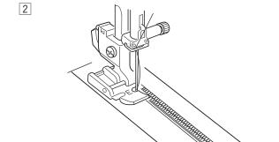
2 Attach the zipper foot E with the pin on the right hand side.
