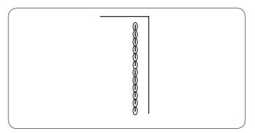
This strong, durable stitch is recommended when both elasticity and strength are necessary in order to insure comfort and durability. Use it to reinforce areas such as crotch and armhole seams. Also use for extra reinforcement when constructing items such as backpacks.
