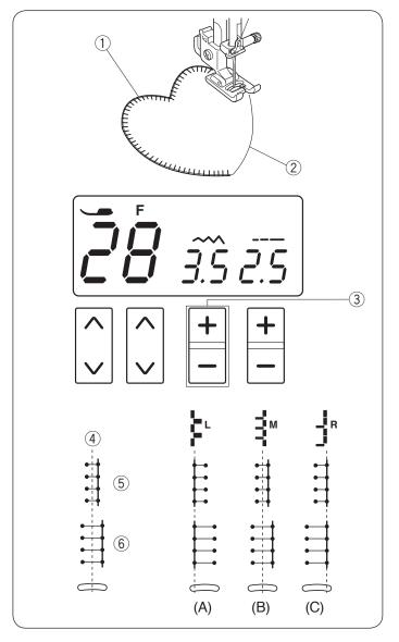
Place an applique on the fabric and baste or pin it in place.
