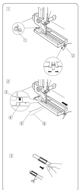
With the buttonhole foot raised, hook the filler cord on the spur at the back of the foot. Bring the ends toward you under the foot, clearing the front end.
