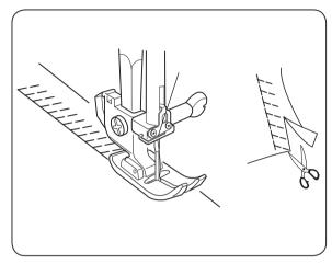
This stitch is ideal for 1/4" (0.6 cm) seams on knits or on medium to heavy weight woven fabrics where you want a narrow seam. It is also great for sewing spandex swim wear. Place the fabric to leave a 5/8" (1.6 cm) allowance. Trim the extra allowance after sewing.
