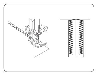
The zigzag stitch is used on the seam allowance to prevent fabric from fraying at raw edges.
