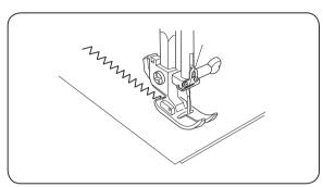
Simple zigzag stitching is widely used for overcasting, sewing on buttons etc.
