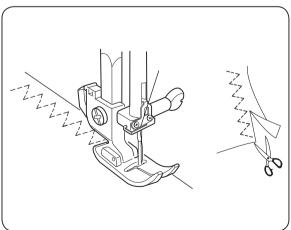
This stitch is used to finish a raw edge on synthetics and other fabrics that tend to pucker. Place the fabric to leave a 5/8" (1.6 cm) allowance.
