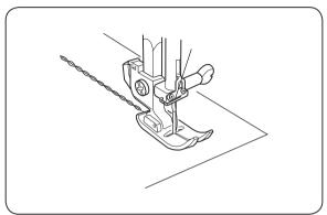
The pattern is sewn with two stitches forward and one stitch backward, forming a seam that does not rip easily.
