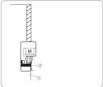
This stitch is recommended for sewing such fabrics as synthetic knits and stretch velour as it provides the greatest amount of elasticity and strength.
