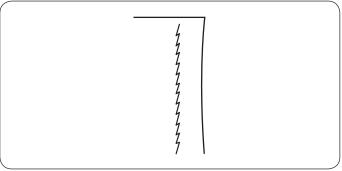
This is a narrow stretch stitch designed to eliminate puckering on knit fabrics and bias seams, while permitting the seam to be pressed completely open flat.
