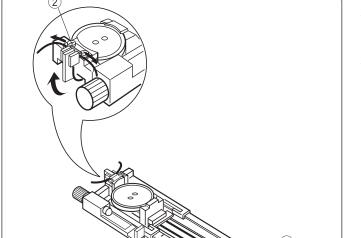
Place the button on the button holder on the buttonhole foot
