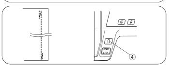
Use this stitch to secure the beginning and the end of a seam with backstitching.
