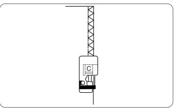
This stitch pattern combines the straight and the zigzag stitches, using the overedge foot, to seam and overcast in one step.
