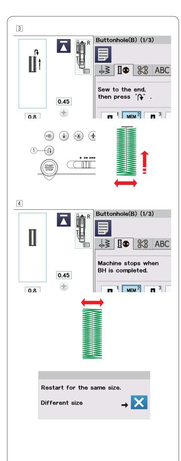
3 Start sewing again, and the machine sews the front bartack and right side of the buttonhole.
