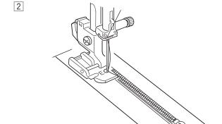
2 Attach the zipper foot E with the pin on the right hand side.
