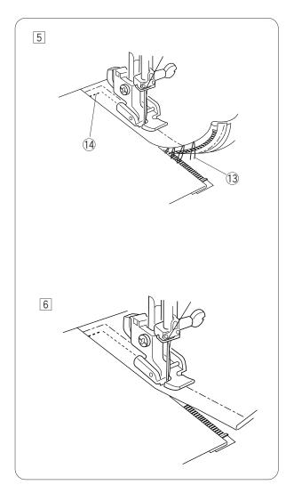
5 Raise and release the foot, and re-attach it with the left side pin.
