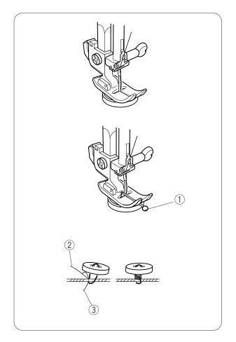
Unthread the needle. Adjust the stitch width to match it with the span of the holes in the button. Turn the handwheel to check if the needle enters into each hole in the button.
