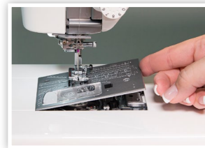
ONE-STEP NEEDLE PLATE CONVERSION
