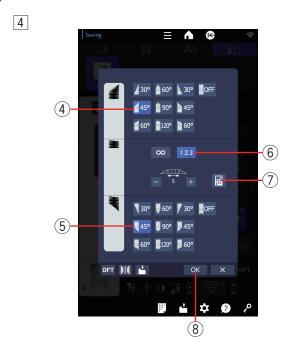
4 Press the tapering shape key (for start tapering pattern) 4.
