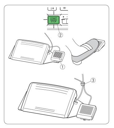
After sewing, depress the thread cutter switch ① on the right side of the foot control to trim both the needle and bobbin threads.
