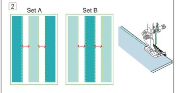
2 Attach 1/4" seam foot O. Stitch the strips right sides together to make strip sets A and B as shown in step 3.
