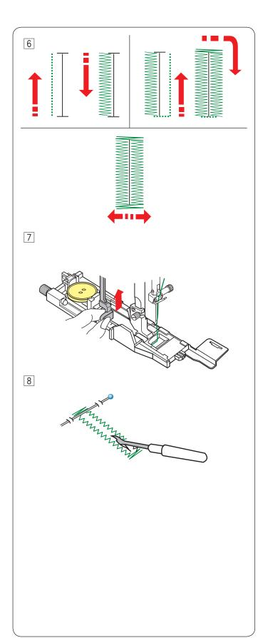
The buttonhole is sewn automatically in the sequence shown. When the buttonhole is finished, the machine will stop automatically with the needle in the up position. Press the thread cutter button and remove the fabric.
